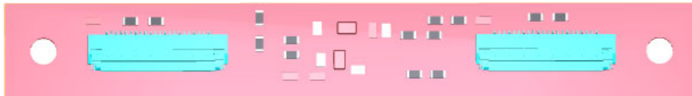
Top View with two camera connectors (J3 and J4)
