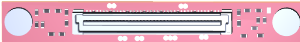
Bottom View with B2B connector (J1)
